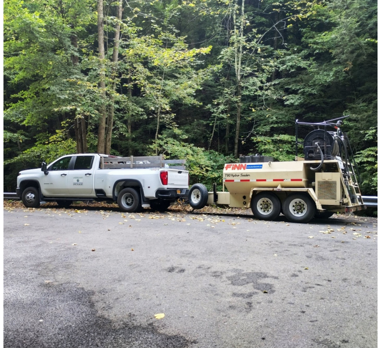
Onondaga County SWCD - Truck and Hydroseeder
